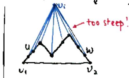
If we place  $v_i$  high enough, then clearly no crossing could occur. But then the slope would be too steep and the invariant breaks. So before actually placing  $v_i$ , we "stretch" the base shape a little. In particular, we shift the portion strictly between  $u$  and  $w$  to the right by unit distance; and the portion from  $w$  to  $v_2$  to the right by distance 2:
